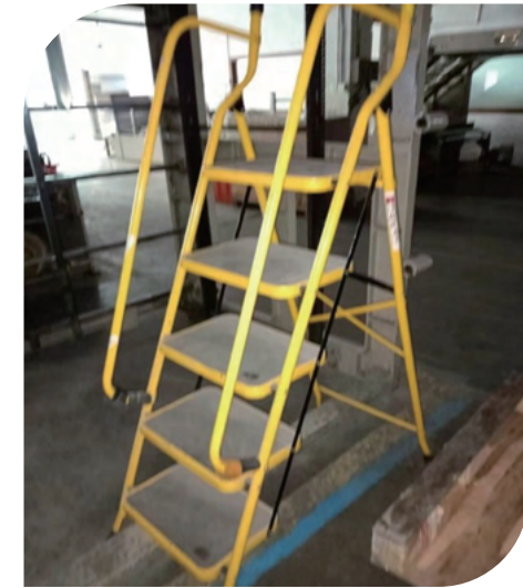
Replacement of a herringbone ladder with a double-sided escalator, which originally posed a risk of falls
